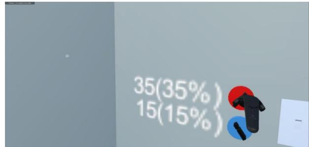
Figure 9: Adaption of the set point temperatures for heating and cooling or switching on/off lights with the dual-stage trigger of the hand controller
