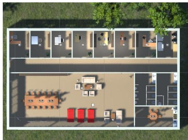
Figure 3: Unity model, enriched with furniture and dynamical building elements (windows, doors, switches). Within Unity the building model was extended with furniture, lights and technical devices, which are
