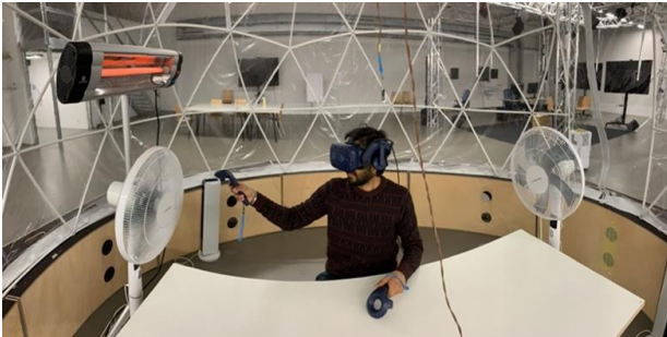
Figure 2: User in the climate chamber of the VR simulation environment: he is wearing a HMD, is doing interaction with the VR building model and is physically getting feedback of the simulated indoor climate
