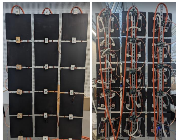
Figure 7: Columns of thermal pixels. left: radiation side; right: back side with TECs and water cooling system
