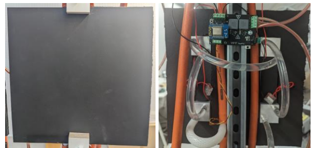
Figure 6: A single thermal pixel (left: front side, right: backside with individual water coolers for each TEC)
